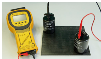
Measurements of surface resistances.
