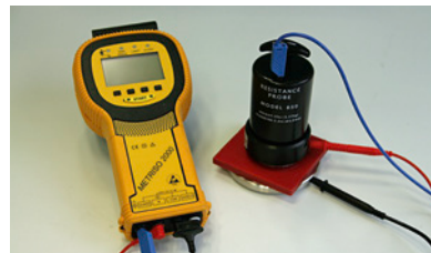
Measurement of volume resistance.
