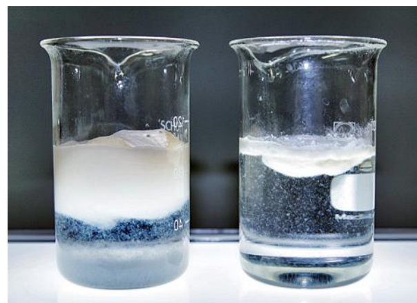
Swelling properties of Deuteron VT 819 (right) and Deuteron XG (left)
